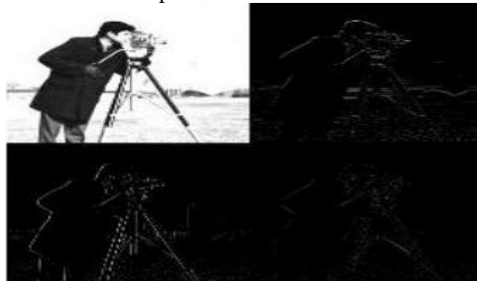
Fig. 2 An I- level 2-D DWT decomposition of Cameraman image
