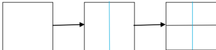
Fig.1 The process of 2-D DWT decomposition
