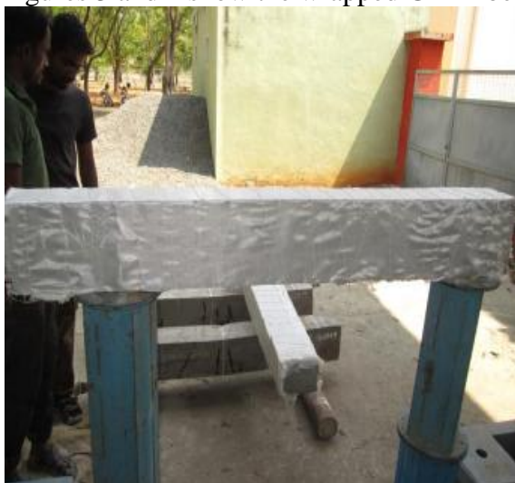
FIG 3 GFRP WRAPPED BEAM - 225GSM
