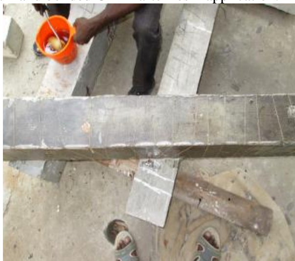
FIG 4 AFTER APPLYING POLYESTER RESIN FOR BONDING – 225 GSM
