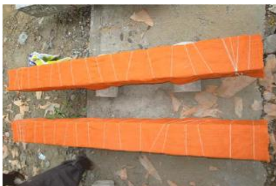
FIG 16 BEAM WRAPPED WITH JUTE FIBER
