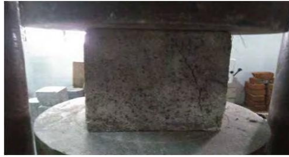
Figure 1 Compressive strength testing of concrete
