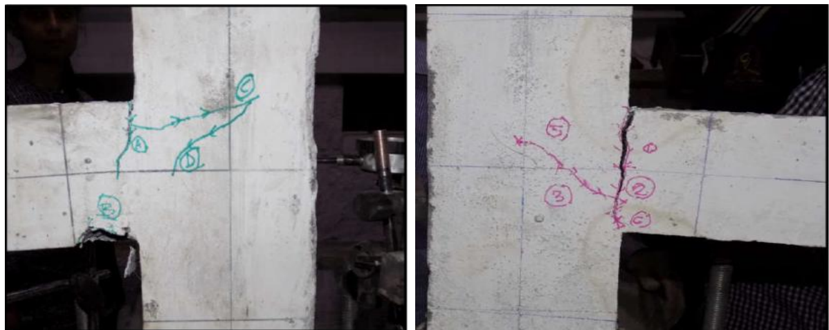
(a) CRACK PATTERN ON FACE A
