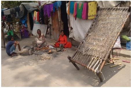
Three members of a loha peet family working as a unit to make tools out of iron. Use of hand fan to keep the bhatti ignited can be located.
