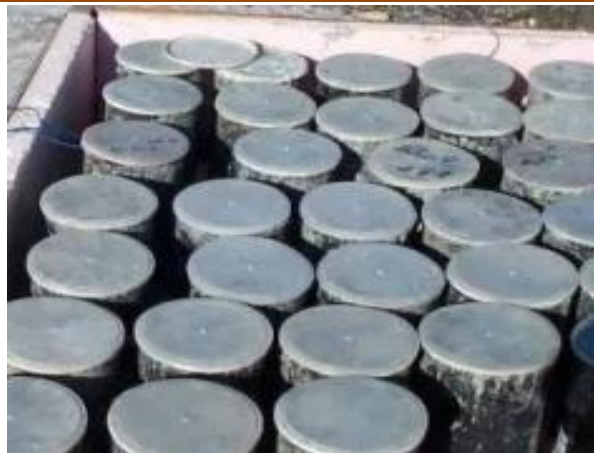
CURING OF SPECIMENS
