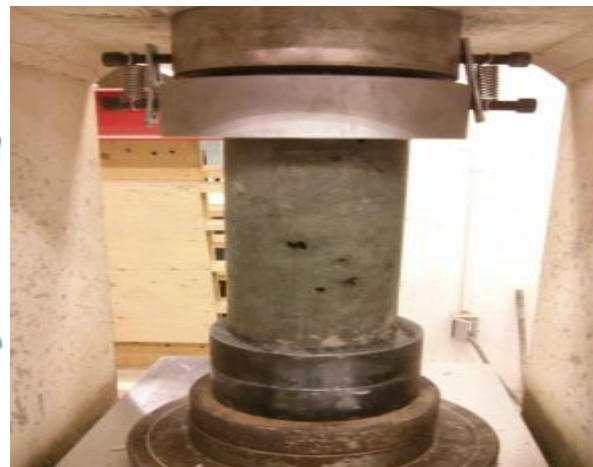
TESTING OF CYLINDER
