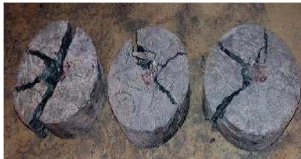
FIGURE 7 IMPACT SPECIMENS AFTER FAILURE
