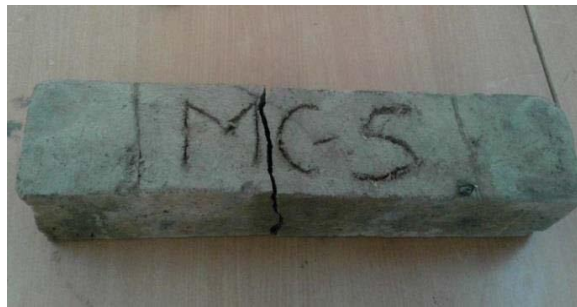
FIGURE 6 BEAMS AFTER TESTING
