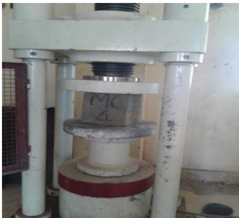
FIGURE 1 CUBES UNDER TESTING SPLIT TENSILE STRENGTH TEST
