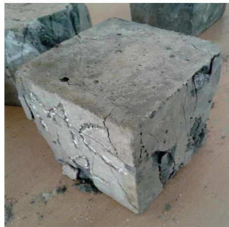
FIGURE 2 CUBES AFTER TESTING
