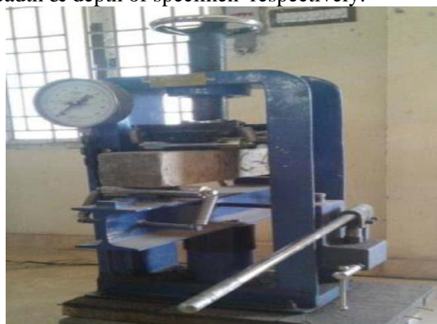
FIGURE 5 BEAMS UNDER TESTING
