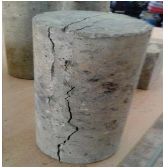
FIGURE 4 CYLINDERS AFTER TESTING
